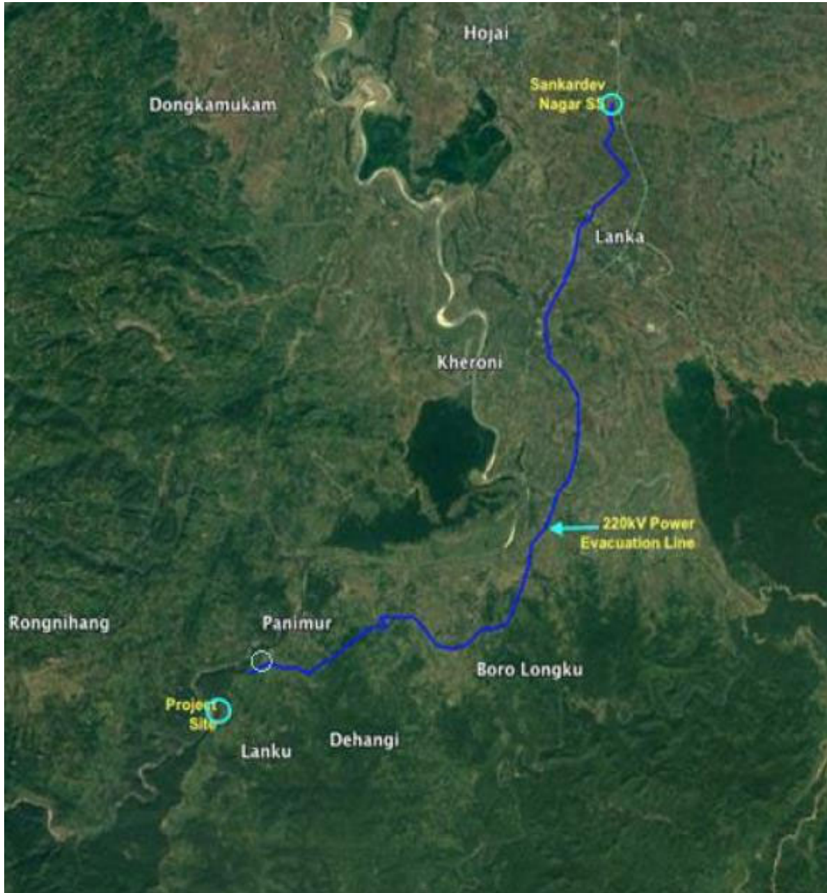
Figure 3: Layout of Transmission line (Google earth)
